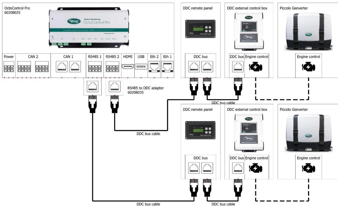
Connect the DDC bus from the generator to either RS485<sup>1</sup> or RS485<sup>2</sup>. Only one generator can be connected per RS485 communication port of the OctoControl Pro. It is recommended to always install the DDC remote panel in the system.
