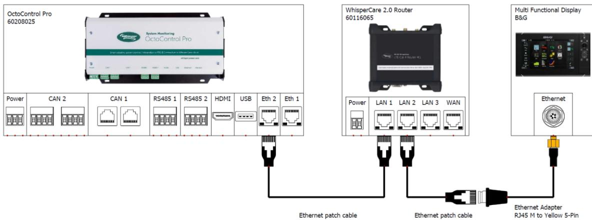
Connect an ethernet patch cable with a Simrad ethernet adapter between the Simrad multi-functional display and the OctoControl Pro. Use the ethernet<sup>2</sup> port on the OctoControl Pro. A WhisperCare 2.0 router is necessary to ensure a functional network.
