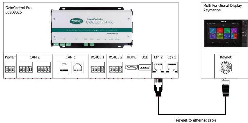
Connect a Raynet to ethernet cable between the Raymarine multi-functional display and the OctoControl Pro. Use the ethernet<sup>2</sup> port on the OctoControl Pro. Follow the instructions of the Raymarine multi-functional display.
