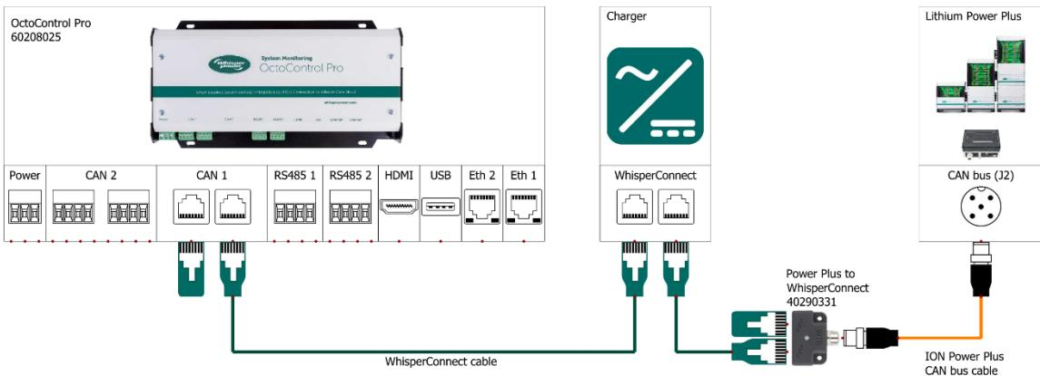
Each Lithium Power Plus battery bank is equipped with a WP-WIB (Whisper Interface Box). This box monitors and provides safety features for the battery bank. It collects and processes all data from each individual battery and presents this information on the CAN bus to be read by the OctoControl Pro. A Lithium Power Plus to WhisperConnect splitter must be used to connect to a WhisperConnect network. CAN<sup>1</sup> must be configured as CANopen in the setup wizard.
