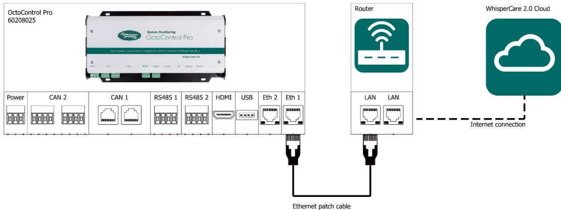
Connecting the OctoControl Pro to the internet allows the use of the WhisperCare 2.0 cloud portal. An energy system can be monitored and controlled using this portal. Furthermore, automatic notifications can be sent in case the energy system needs attention.
