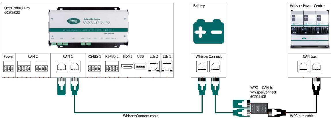
WPC bus can be connected to the WhisperConnect bus via the WPC-CAN interface. Follow the instructions in the WhisperConnect segment. CAN<sup>1</sup> must be configured as WPC bus in the setup wizard.
