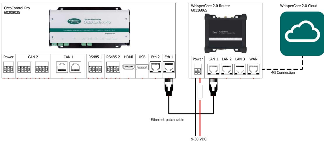
When no internet connection is available a WhisperCare 2.0 4G router can be used. Connect an ethernet patch cable between the OctoControl Pro and the WhisperCare 2.0 4G router. Use the ethernet<sup>1</sup> port on the OctoControl Pro. Install the sim card into the router. Configure the router following the WhisperCare 2.0 4G router manual.
