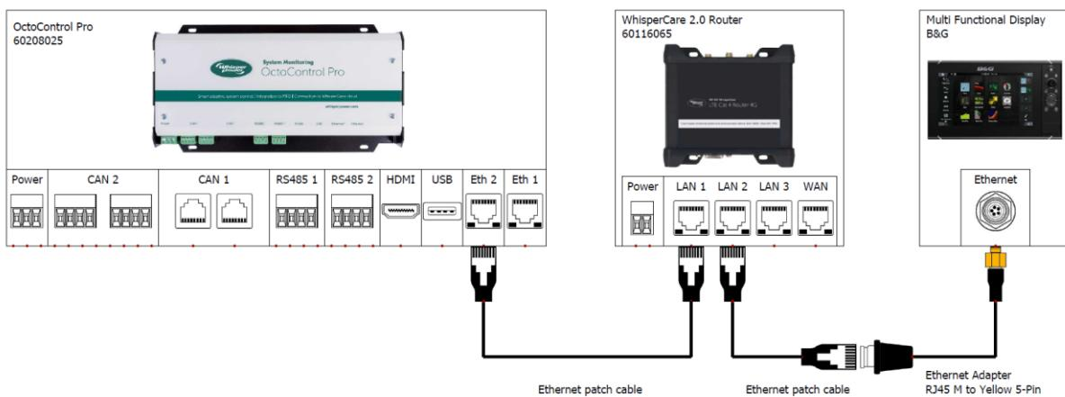
Connect an ethernet patch cable with a B&G ethernet adapter between the B&G multi-functional display and the OctoControl Pro. Use the ethernet<sup>2</sup> port on the OctoControl Pro. A WhisperCare 2.0 router is necessary to ensure a functional network.
