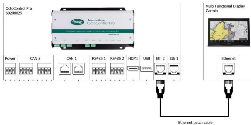
Connect an ethernet patch cable between the Garmin multi-functional display and the OctoControl Pro. Use the ethernet<sup>2</sup> port on the OctoControl Pro. Follow the instructions of the Garmin multi-functional display.
