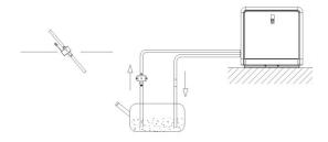
Figure 5: Fuel line assemblies with pump mounted vertically or in an angle
