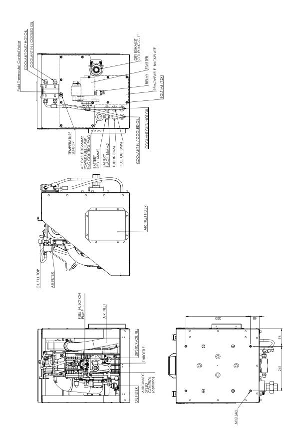
Figure 13: Main components and mounting rectangle
