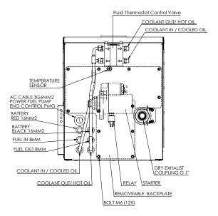
Figure 2: Genverter connections
