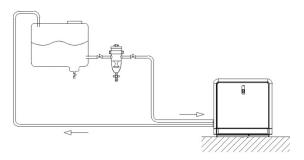
Figure 4: Fuel tank above the genverter
