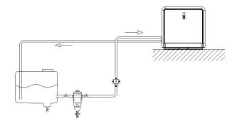
Figure 3: Fuel tank below the genverter
