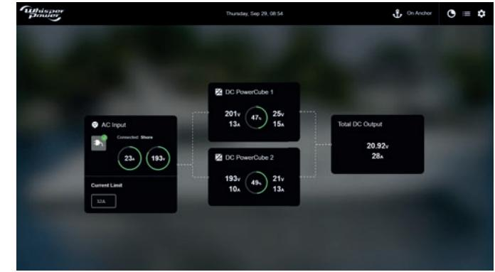
Summarized input and output power data combined from all chargers in a system
